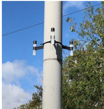
Figure 1: Diffusion tubes installed in triplicate at a site in the Parish
